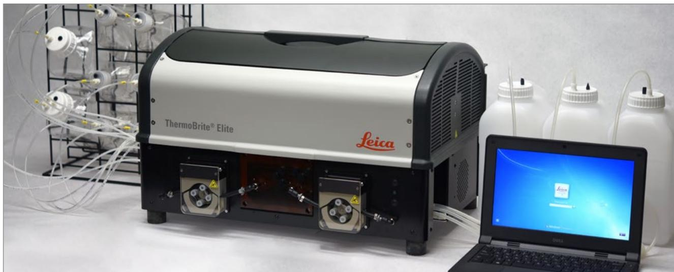
The ThermoBrite Elite automates and standardizes the FISH slide preparation process including deparaffinization, pretreatment, denaturation/hybridization and post hybridization wash. Application of probe, counterstain and cover slipping are the only manual steps. Just load your slides and walk away. Minimal hands-on time frees up technologists for other important tasks.
