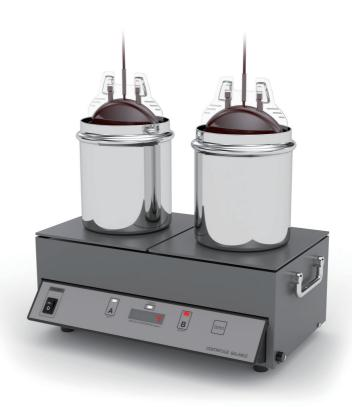
\*B-side is lighter by 4 grams. Adding a few weight-chips in B will make GOOD lamp light.
